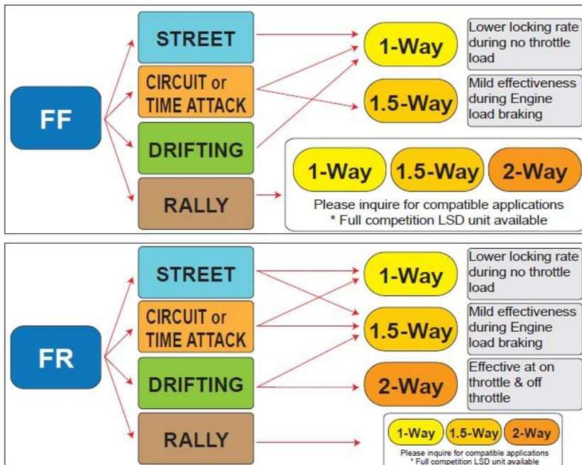
To change the "way" of the LSD for example from a 1.0 to a 1.5 you have to open the LSD. To do this remove the screws and pull the two sections apart. Once open, revolve the cam/adaptor to the position shown in the diagram below. The cross-pin needs to have the rounded part pointing the opposite way to the diffs
