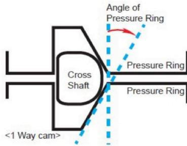
Initial preload is around 85lb. To change the preload, you need to remove or add springs, (there must be equal numbers i.e. 4, 6, 8, 10, 12). Unfortunately, the only way to check the preload value is to use a torque wrench with a special tool that is inserted into the LSD (like an axle shaft). This is available for purchase separately. The more preload you have, the less the LSD will slip under low torque conditions. (6 springs will provide approximately 55lbs)
